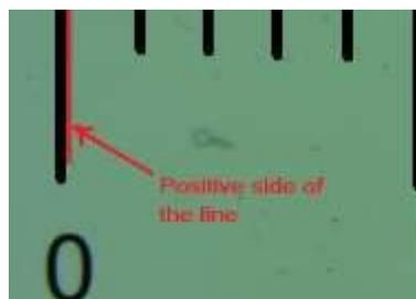
Length 1 - Measure the zero line and the Length 1 measuring line on the glass scale and construct a distance between the two lines.
