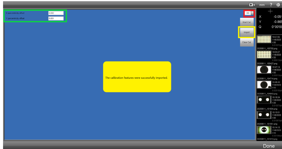
Figure A9 – Successful parcentricity correction
